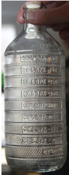
Clear bottle embossed "Knurl & Stipple Guide" with various numbered examples of knurling and stippling around the bottle
