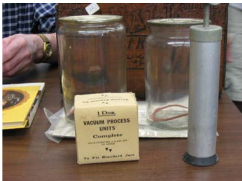
Vacuum Seal jar and all of its original go-withs. The pump was used to create the vacuum.
