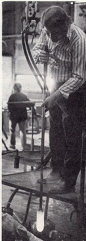
...who completes the shaping, forms the jar, and "blows the straw."
